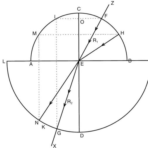
**Fig. 7. Mydorge's Refraction Prediction Device**
