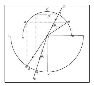
Figure 5. Mydorge's Refraction Prediction Device
